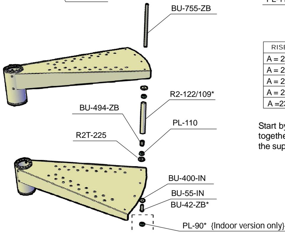
To assemble the through columns correctly, follow these steps (1,2,3,4).
