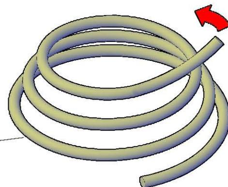
Unwind the plastic handrail according to the upward direction, trying to give it a helical direction similar to that of the staircase.
