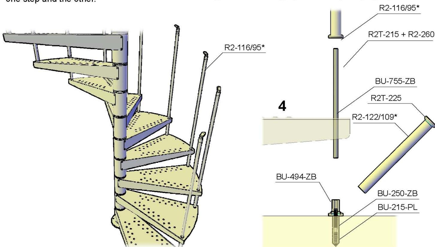
Complete the assembly of the intermediate columns using the sequence shown in the table on page 10, fixing them to the slotted hole of the step, by means of a screw code BU-55-IN (oBU-42-ZB\*) and washer code BU-400-IN.
