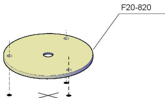
To place the pole correctly, use the starting plate as a "template" and center it with respect to the X previously marked on the floor that determines the center of the staircase (see page 2).
