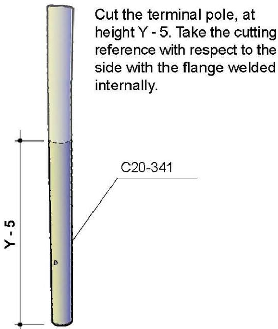
Cut the terminal pole, at height Y - 5. Take the cutting reference with respect to the side with the flange welded internally.
