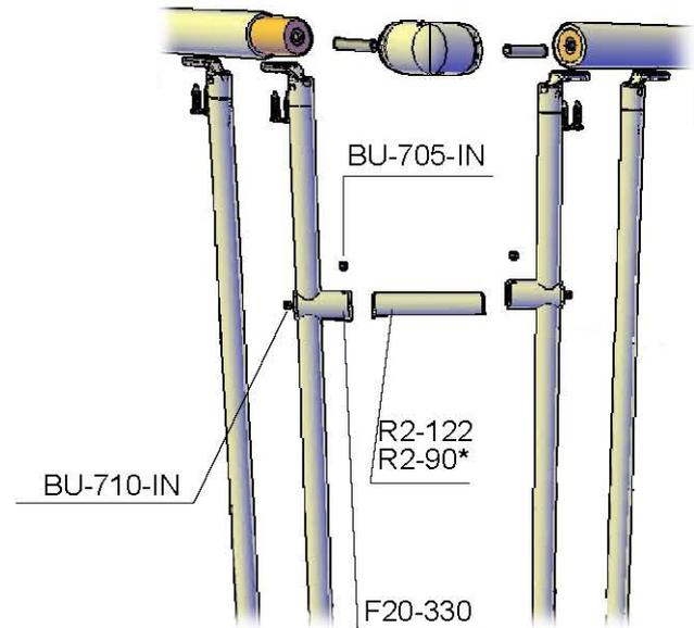
Cut the joint R2-122/90\* to the useful length and secure it to the columns, as shown in the figure.
