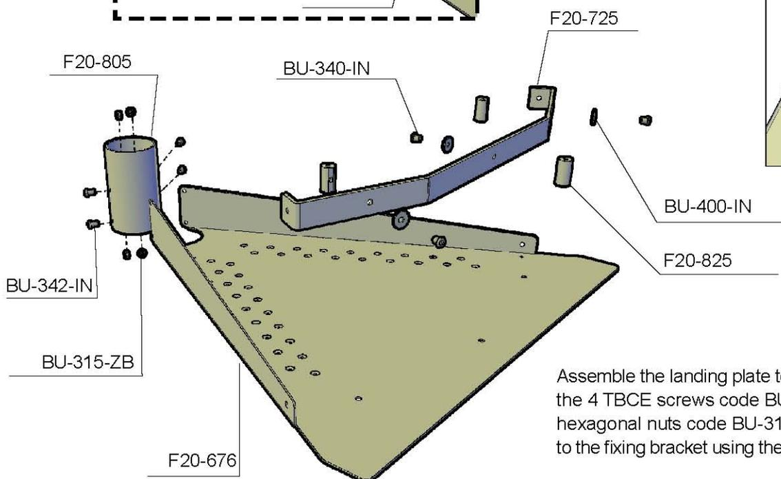
Assemble the landing plate to the relative tubular, using the 4 TBCE screws code BU-342-IN with the M8 hexagonal nuts code BU-315-ZB. Attach the 3 pawls to the fixing bracket using the relative screws, as shown.
