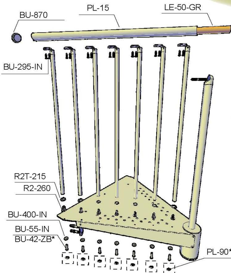
Secure the  $\varnothing 91$  columns code R2-116/95\* of the balustrade in the  $\varnothing 9$  mm holes, using the appropriate bolts.
