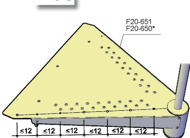
Draw a line with the pencil from the centre of the staircase to the hole F. Drill as many holes as necessary to apply the balustrade columns, drilling with a  $\varnothing 9$  mm drill, maintaining a spacing as per the drawing.
