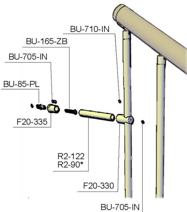
The column - wall joint can also be used on the staircase, as an alternative to the step rivet.
