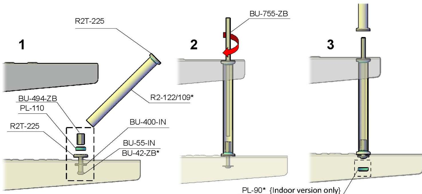
**1)** Insert all the bolts and the PL-110 and R2T-225 accessories (whose number varies according to the lift) in the hole at the back of the step, without tightening permanently. Introduce the support from the external side of the staircase, in the space between one step and the other.
