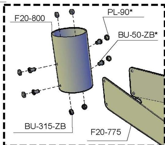
In the indoor staircase version, the TPCE screws code BU-50-ZB and related screw caps are used, as highlighted here.
