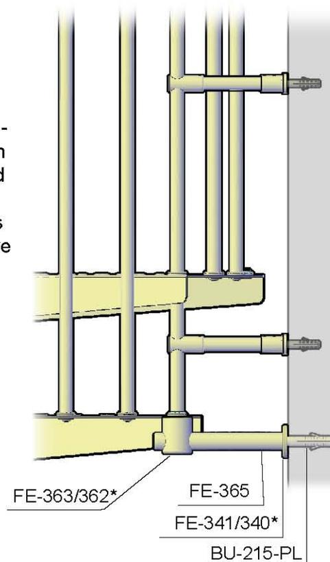
**N.B.:** All cuts and holes made in the outdoor staircase version must be protected with silicone.
