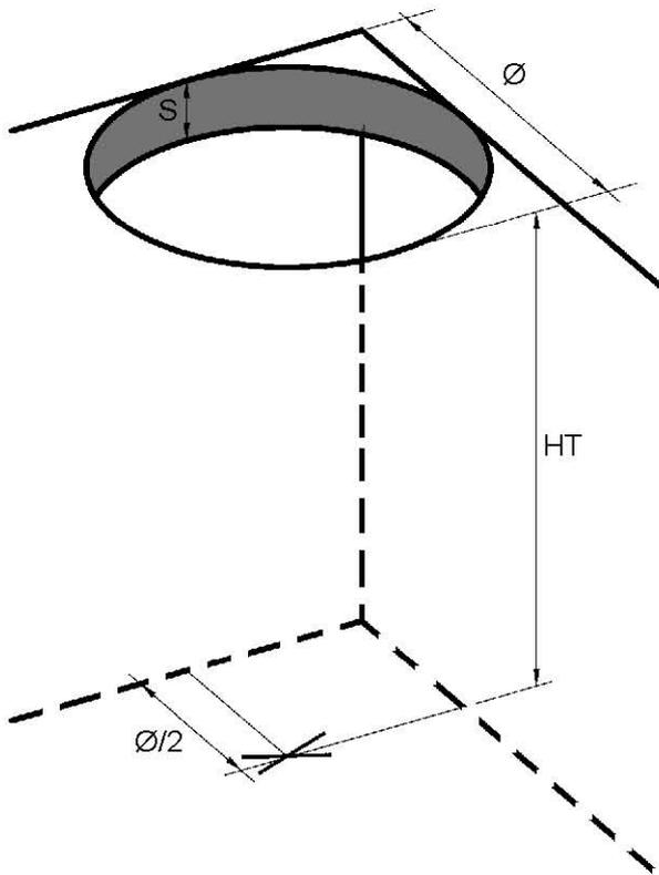
Check the dimensions of the stairwell and the total height, comparing them with the project. Using heights, locate the exact center of the staircase, and mark it on the floor.
