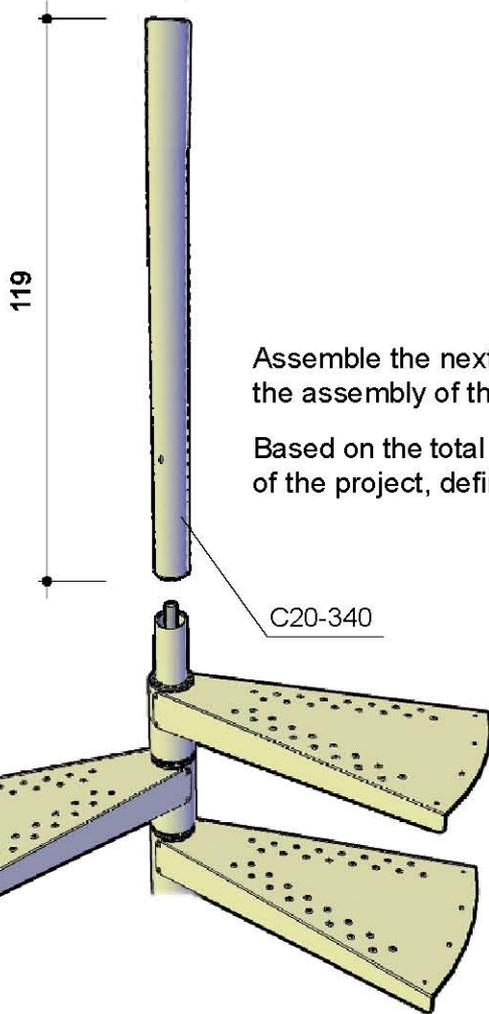
Assemble the next poles and continue with the assembly of the steps.
