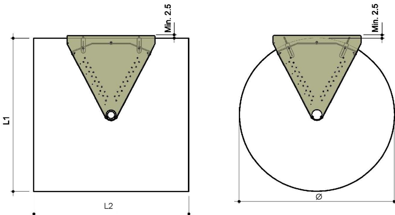
The landing step, suitable for both square and round holes, must be placed in contact with the floor above, leaving a minimum overlap of 2.5 cm.
