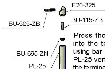
Press the BU-695-ZN element into the terminal core F20-320 using bar BU-115-ZB. Mount the PL-25 vertical plastic handrail in the terminal, backing up the flange. Tighten everything with the end element code F20-325.
